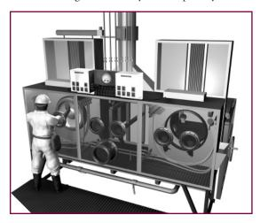
designed sealed glove box system that has been safely used by the Army and the chemical industry for more than 40 years. A tube is inserted into the container and the agent is pumped to an agent holding tank.
