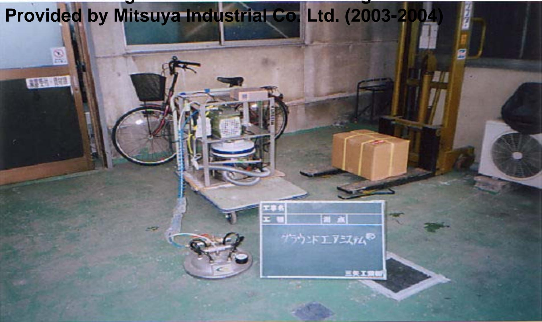
**1 m-depth Core Boring for Soil Gas Investigation
