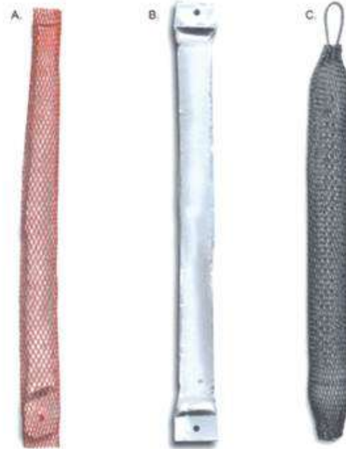
A: Diffusion Bag with Polyethylene Mesh B: Diffusion Bag Without Mesh C: Diffusion Bag and Mesh Attached to Bailer Bottom
