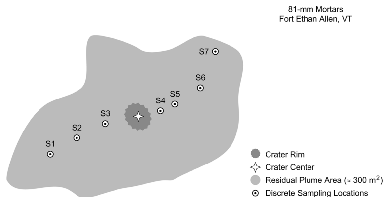
Figure 1. Residue plume from the blowing in place of 81-mm mortar round with a block of C4, with sampling and crater locations marked.
