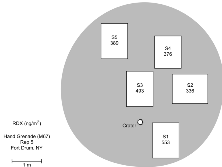
Figure 5. Residue plume #3 from the live-fire detonation of M67 hand grenade with the surface area sampled and concentrations of RDX determined.
