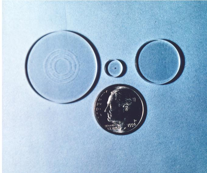
**Figure 5.** FO-LIBS Sapphire Windows (Larger Window Shows Concentric Ablation Pattern Generated by Moving the Laser Pulse Across the Window)
