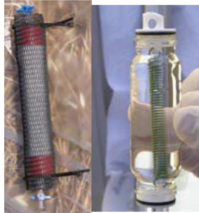
Left: RPP Sampler; Right: Snap Sampler
