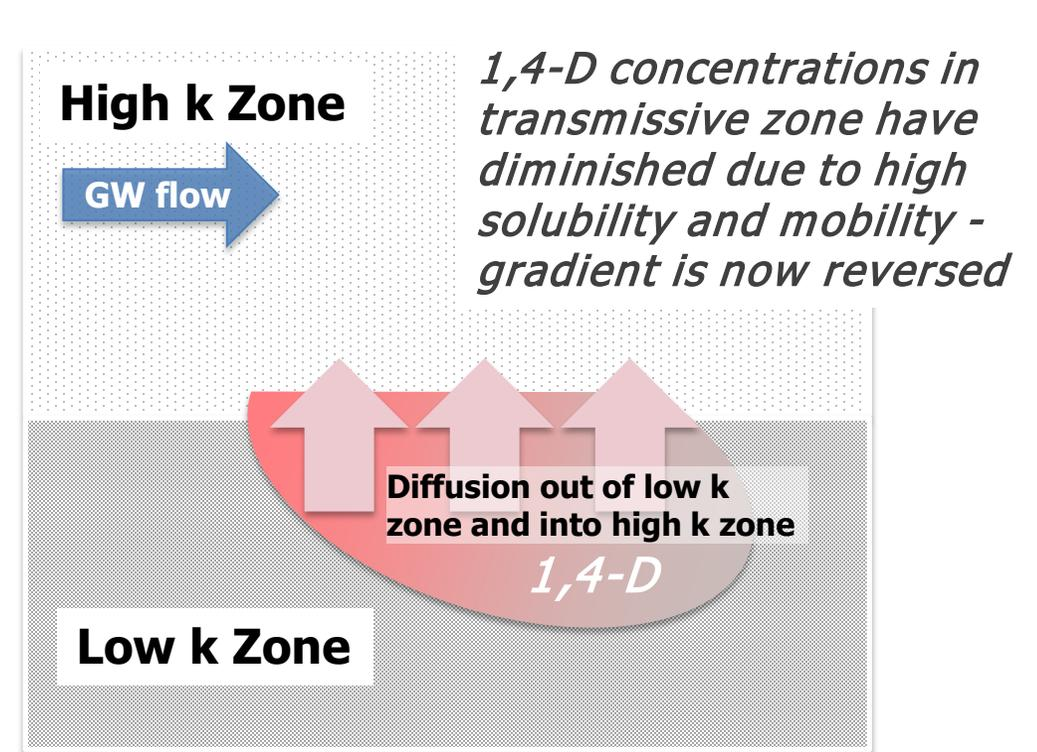
Figure 3-2. Overview of Matrix Diffusion Process for 1,4-Dioxane.
