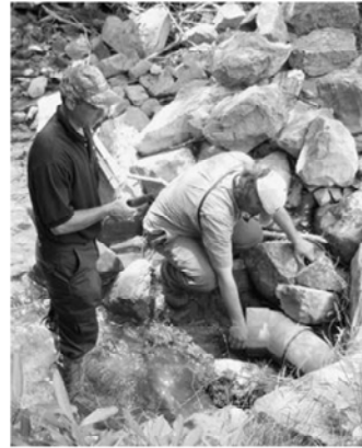
Effluent pH and Eh Testing
