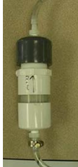
Column used to collect perchlorate for CSIA
