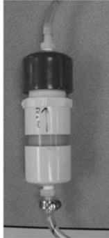
**Column used to collect perchlorate for CSIA**
