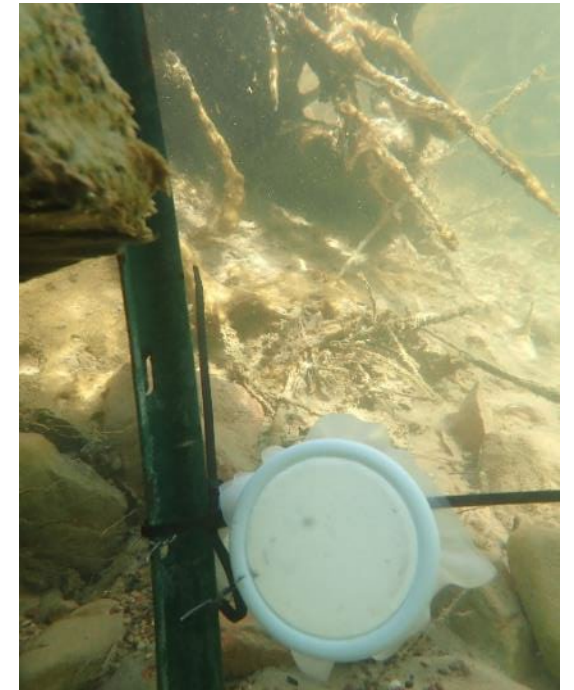
Fig. 4-12. Deployment of a SPATT sampler for cyanotoxins in Zion National Park. Source: Robyn Henderik, used with permission.
