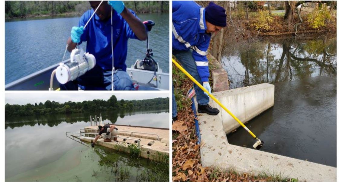
Fig. 4 – 9. Examples of several ways to collect grab samples for cyanobacteria. Source: NJ DEP, used with permission.
