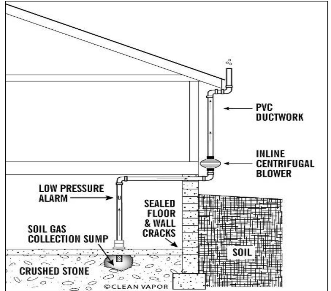
Figure 1 of the Sub-slab Depressurization (SSD) Technology Information Sheet.
