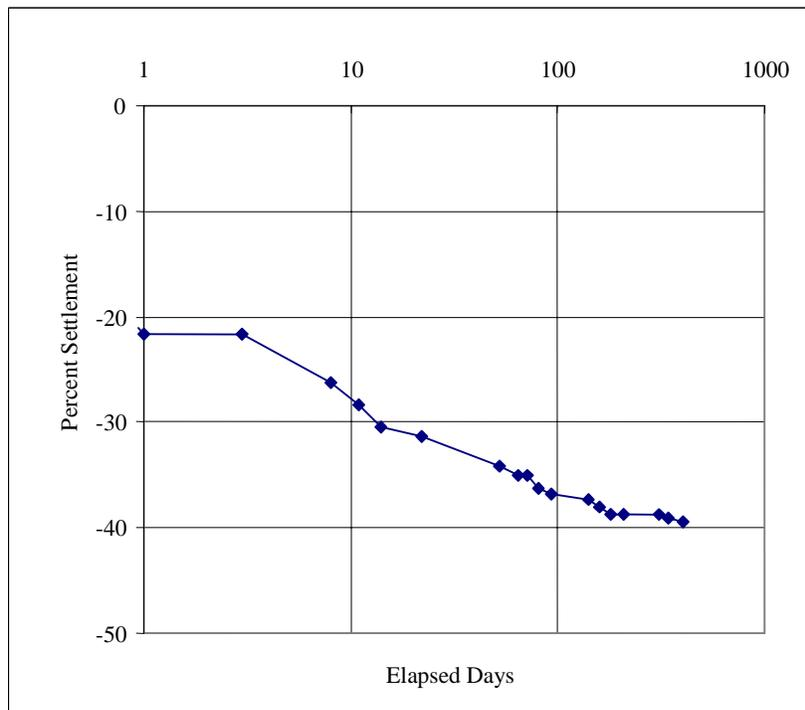
**Figure 3-2. Liquids recirculation settlement results after moisture addition to field capacity of MSW (Pohland, 1975)**
