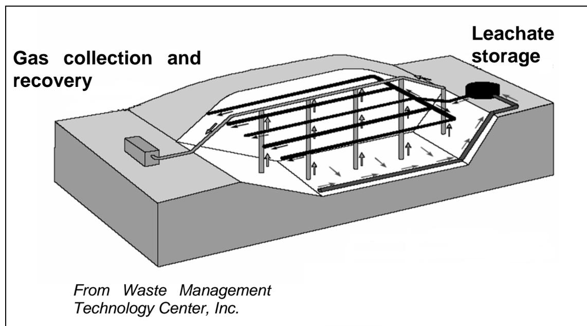
**Figure 3-5. Leachate injection and gas recovery system**
