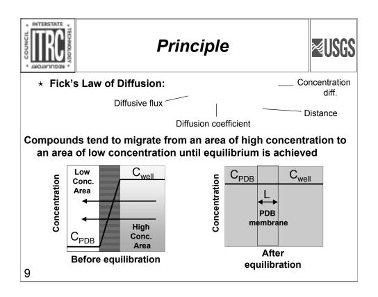
Passive Diffusion Bag (PDB) samplers rely on the mass transfer of dissolved gasses through a polyethylene membrane. The rate of diffusion is described by Fick's Law, shown here, which, in simple terms, states that compounds tend to migrate from an area of high concentration to an area of low concentration until equilibrium is achieved. In the case of PDB samples, the VOCs migrate through the membrane into the sampler until the concentrations are the same on both sides of the membrane.
