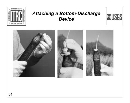
The water also can be removed from the PDB sampler by attaching a bottom-discharge device.
