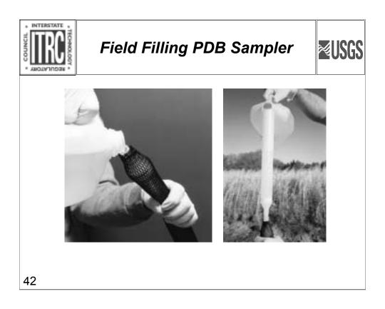
The unfilled samplers can be filled in the field by pouring deionized water into the sampler directly or through a funnel (provided).
