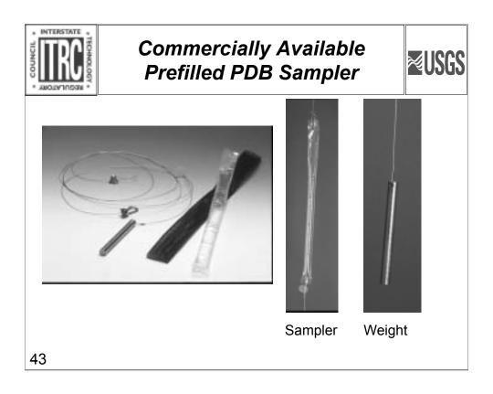
PDB Samplers also are available prefilled with laboratory-grade deionized water.
