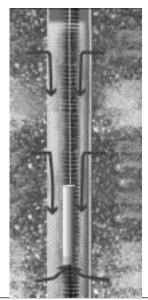
When a pump is turned on, water enters the well through all permeable zones and moves toward the pump.
