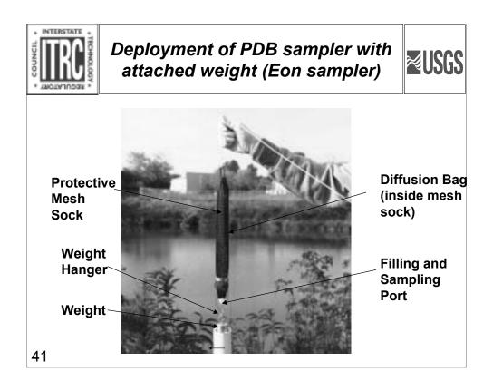
This is an example of one of the types of commercially available PDB samplers. This one is supplied unfilled and can be filled by the user.
