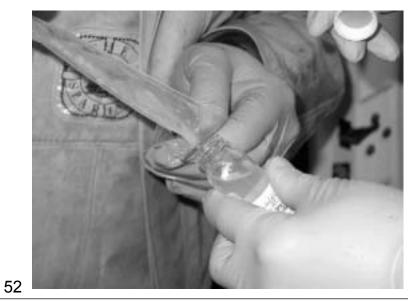
Water also can be recovered from the PDB sampler simply by cutting open with a clean pair of scissors and pouring it into vials in a manner that minimizes agitation. Good comparisons to conventional sampling have been shown using all three water-transfer methods.
