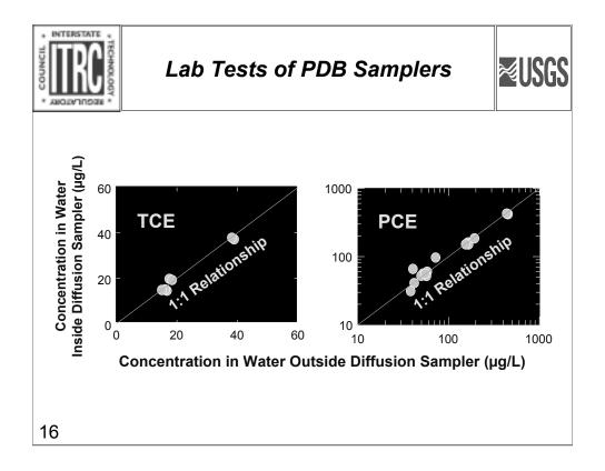
Shown here are some laboratory data for trichloroethene (TCE) and tetrachloroethene (PCE) showing a close comparison of concentrations between water inside and outside the PDB samplers for a range of concentrations.
