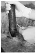
Inserting the tube through the polyethylene into the PDB sampler
