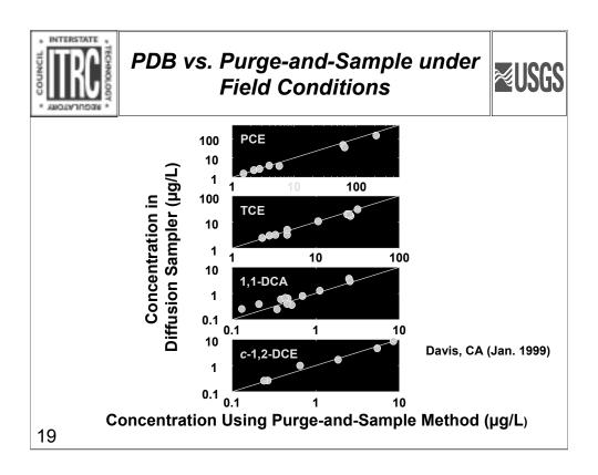
When compare VOC concentrations from PDB samplers under field conditions to VOC concentrations from pumped samples, we usually see a close relation. In this case, the comparison is made to a purge-and-sample methodology.
