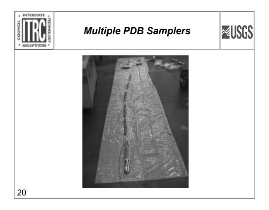
To examine the potential for heterogeneity in wells, we can use multiple PDB samplers attached to a weighted line. There are a number of factors in a screened interval or open borehole that can cause mixing and make a uniform concentration within the screened interval despite the presence of stratification in the aquifer. These include dispersion, in-well vertical flow, and thermal convection.
