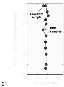
In some wells, there is no stratification, indicating in-well mixing. A close match is observed between the low-flow sample and the PDB samples.
