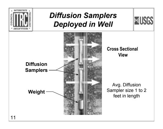
That is where the diffusion samplers come in. PDB samplers are deployed in the screened interval and allowed to equilibrate. After sufficient equilibration, the samplers are removed and the enclosed water is transferred to volatile organic analysis (VOA) vials. Thereafter, the samples are treated as ordinary VOA samples.
