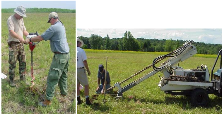
Using an auger and a post hole digger to emplace seed items on a test plot
