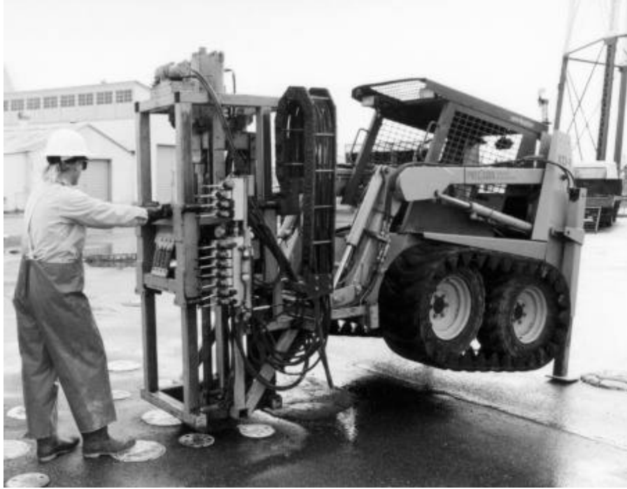
Figure 8-10. Enviro-Core™ Sampler Extracting Angled Core at Former NAS Moffett Field
