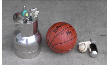
Examples of sampling canisters (shown with sporting equipment to illustrate size)
