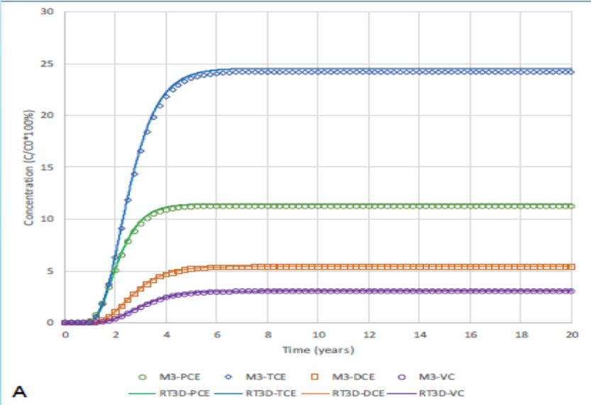
Comparison of Model 1 to MT3DMS, source duration 10 years, dual porosity
