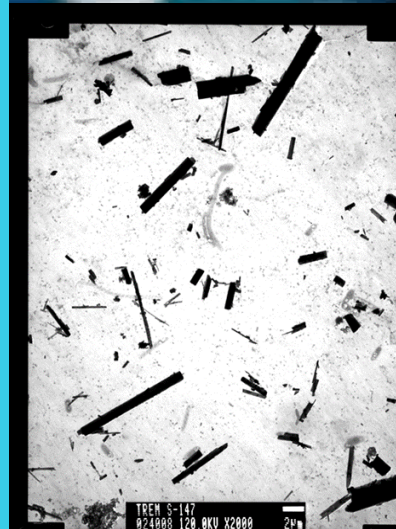
Asbestos RARE Project, SFP-131B Sample Number 18154000 400x, Phase Contrast FBAS, 0.5-gram test Jed Januch, 9/23/2020
