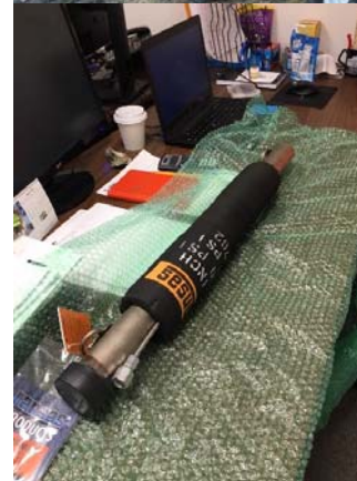
Packer in HDD wells to focus sparge in distal well end
