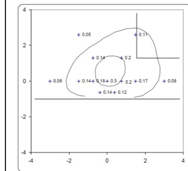
Uplift above Fractures T3 and T4. Uplift measured at locations indicated by + and recorded in cm. Axes indicate north / south and east / west distances in meters from center of uplift array. Contours shown for 0.1, 0.2, and 0.3 cm of uplift. Perimeters of the cellar, steps, house, and outbuilding indicated by light straight lines.
