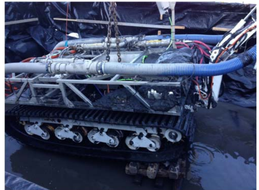
Photograph 13: Sediment located within the inside of the Scancrawler (10/21/2013)
