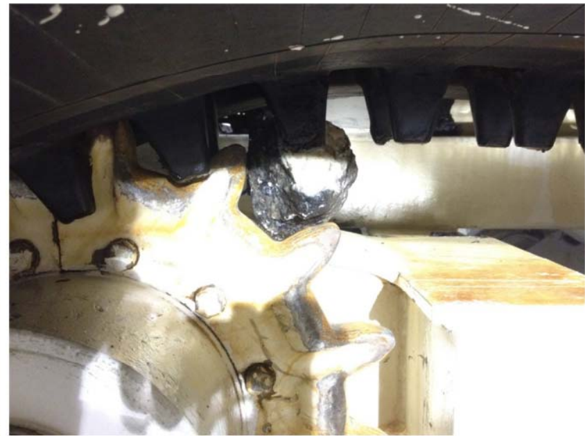
Photograph 3: Rock stuck in the track of the Scancrawler - preventing movement of equipment (10/10/2013)
