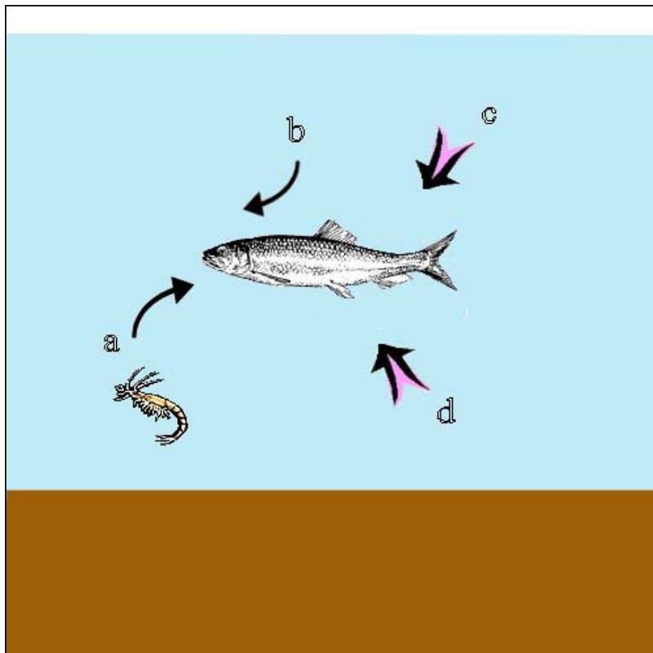
*Figure 2-2 Exposure pathways for aquatic organisms as considered by FASSET. (a) Internal exposure via ingestion of contaminated food and assimilation; (b) internal exposure via direct uptake from the water column; (c) external exposure directly from radionuclides in the water column; (d) external exposure from radionuclides in sediments.*
