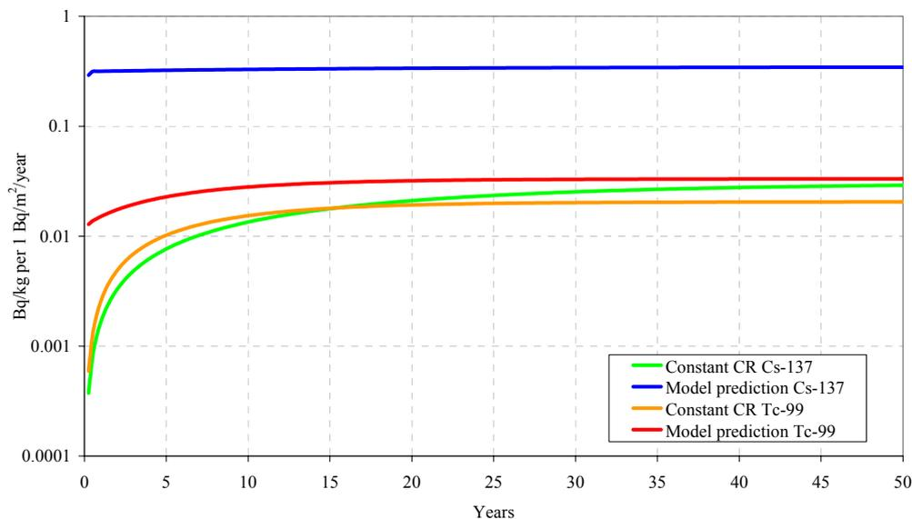
Figure 4-1 Predicted  $^{137}\text{Cs}$  and  $^{99}\text{Tc}$  activity concentrations in a 1.75 kg herbivorous mammal assuming a constant annual deposition over 50 years. Predictions assuming an equilibrium soil - reference organism CR over the simulation period are compared with predictions using the dynamic model described in Appendix 2 (Section 5).
