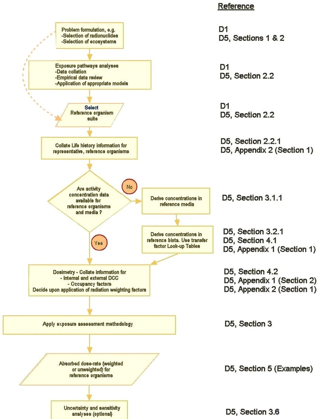
Figure 1-2 Flow diagram showing stages in the FASSET exposure assessment
