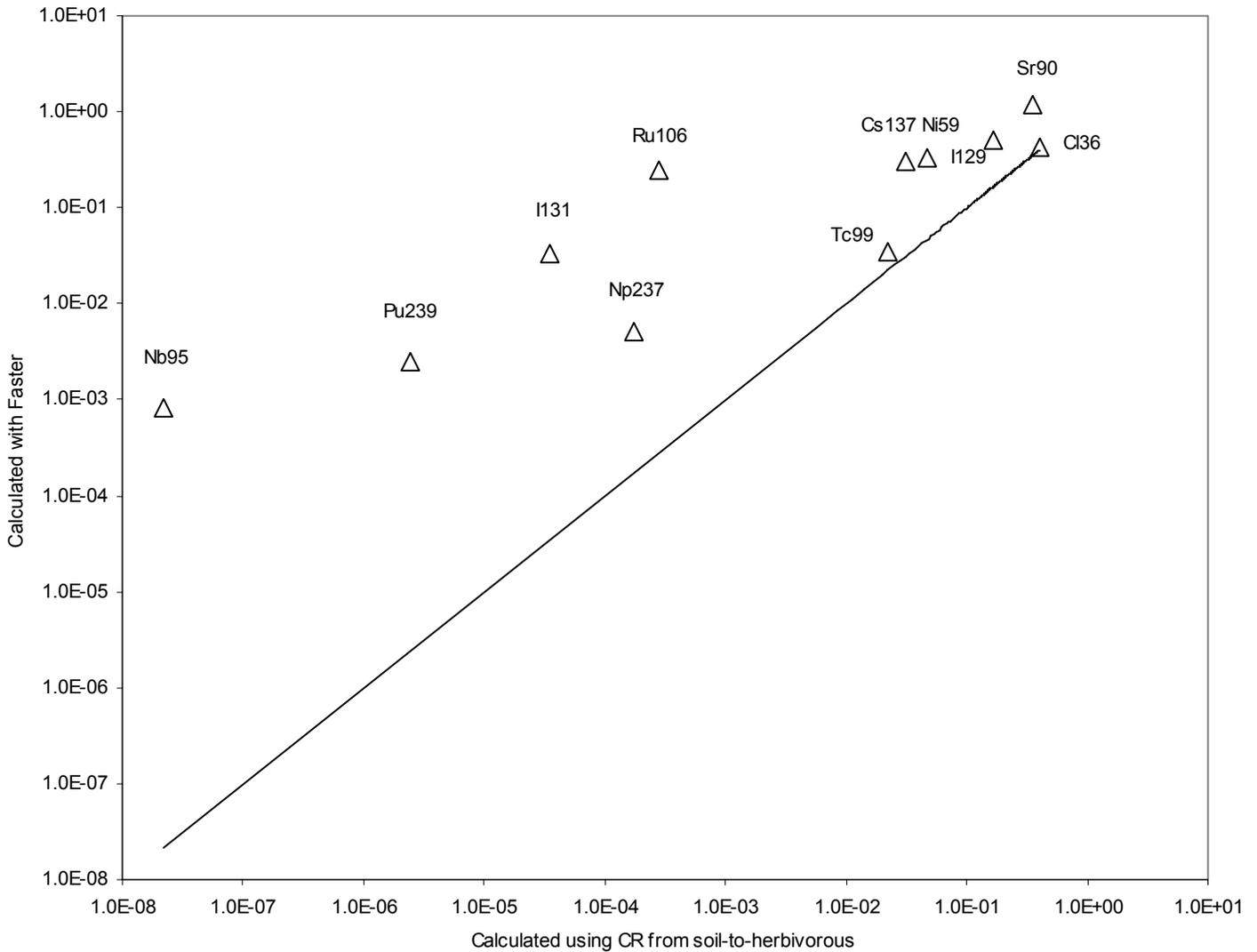
Figure 3-4 Activity concentrations in herbivorous mammals after a continuous constant deposition of 1 Bq/(m<sup>2</sup>y) above a semi-natural ecosystems calculated with the computer program FASTER (Appendix 2, Section 5) and with the CR in the look-up tables under Section 1.2 in Appendix 1. For radionuclides with low soil-to-plant CR the use of CR leads to underestimation of the activity concentrations in herbivorous mammals.
