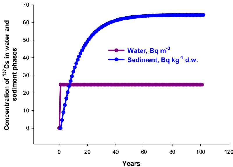
Figure 5-1 <sup>137</sup>Cs dynamic concentrations in the marine environment following a 1TBq release to a generic compartment.
