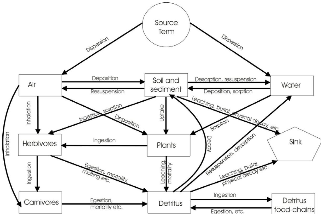
Figure 2-1 Processes affecting radionuclide behaviour in ecosystems (Based on Whicker & Shultz, 1982).
