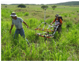
EM61-MK2 used in DGM (left) and "mag and dig" (right) modes. Photos courtesy of US Navy.
