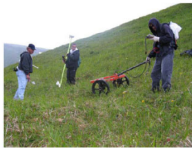
EM61-MK2 used in DGM (left) and "mag and dig" (right) modes. Photos courtesy of US Navy.
