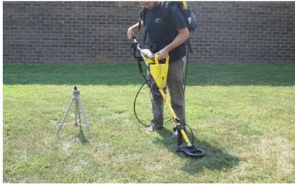
**Electromagnetic methods:** An **active** detection method that generates a signal, which in turn, induces buried metal to generate a magnetic field
