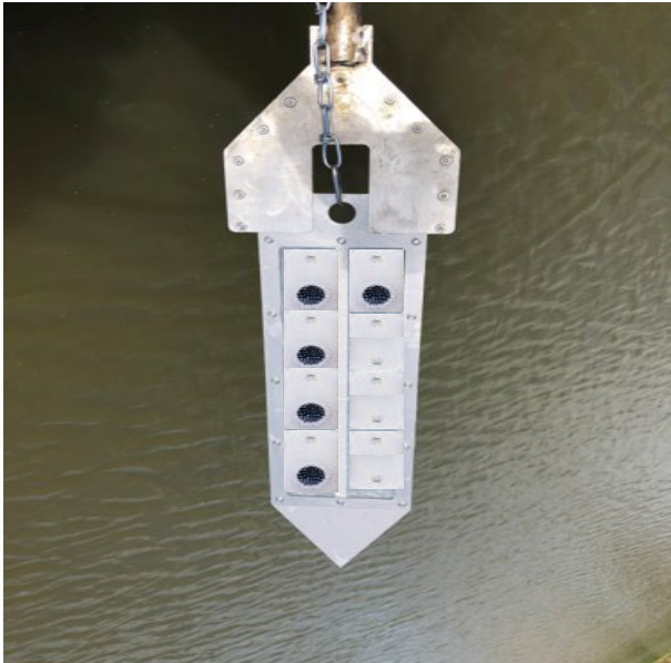
Conceptual prototype frame for deployment of array of passive samplers in sediment.
