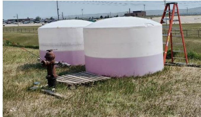
Mixed Tanks for Stream Tracer Test
