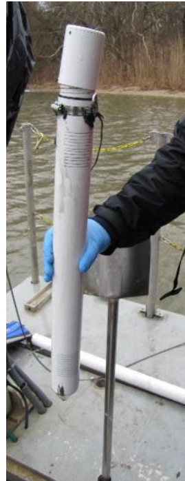
Schematics and photo of the SBPVP (Cremeans and Devlin, 2017). SPVP photo courtesy Rick Devlin
