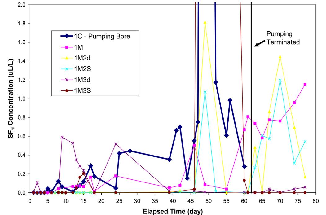
SF<sub>6</sub> Tracer breakthrough in pumping and monitoring wells
