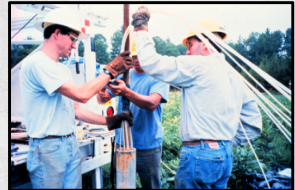
Tubing, electrical connections for downhole sampling equipment
