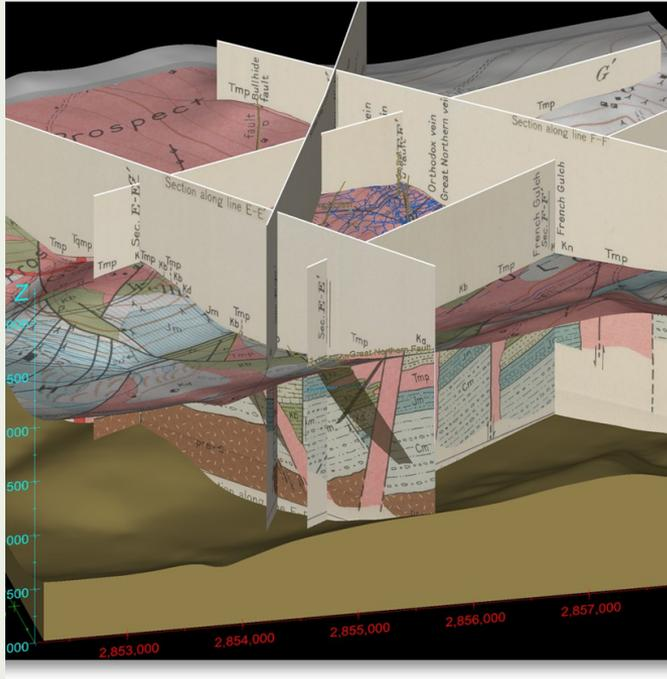
Placing cross sections and mine level maps in correct orientations
