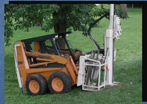
Direct Push Unit Powered by Skid Steer
