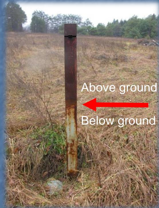
Outer casing found loose enough to be lifted out of ground
