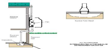
This shows suction point close to basement wall. Note that we always try to put these in the center of the home where possible – some do end up against the wall, but it's not typical
