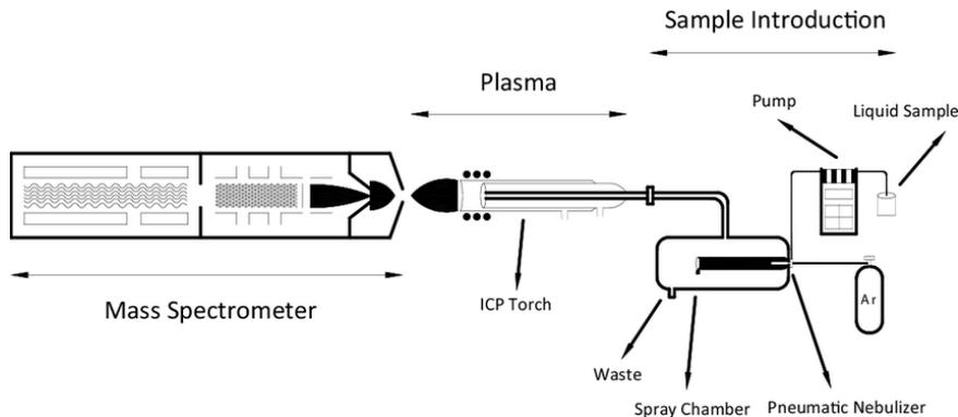
Figure 1: IC-MS diagram
