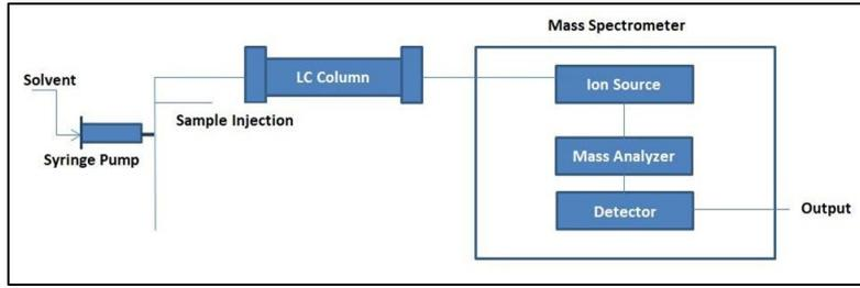
Figure 2: LC-MS diagram
