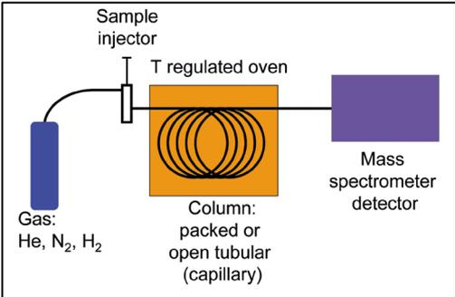
Figure 1: GC-MS diagram
