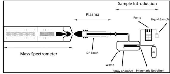
Figure 4: IC-MS diagram
