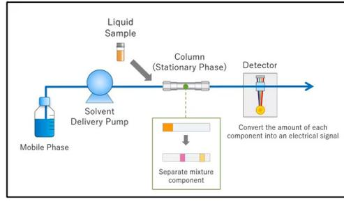
Figure 3: HPLC diagram
