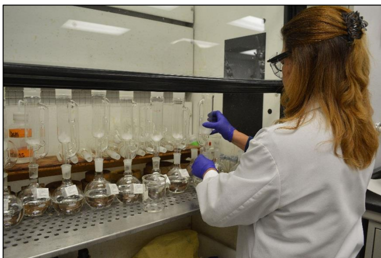
Chemist setting up solvent extraction equipment in a fume hood.
