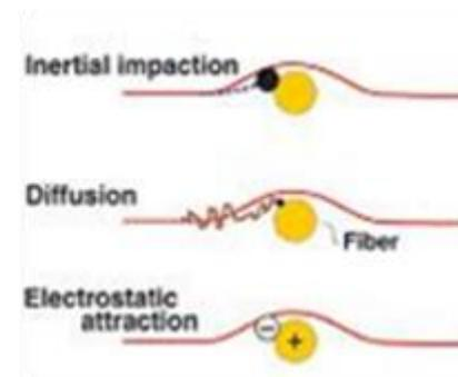
Filter efficiency mechanism
