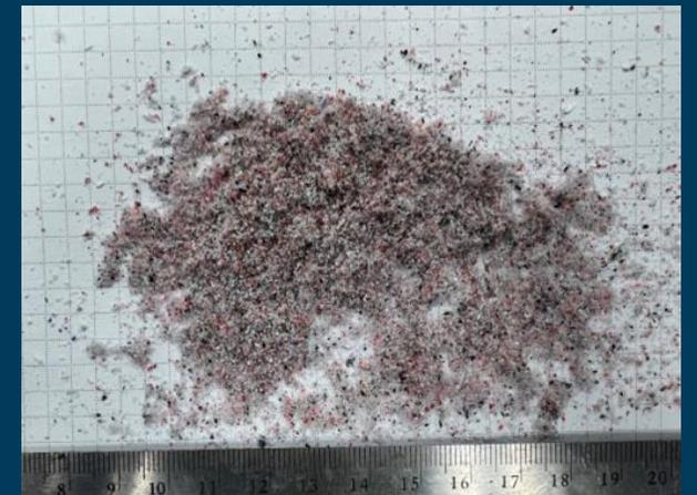
HDPE plastics before (top) and after being milled through a 0.50mm sieve ring (bottom). (*From Fritsch Milling & Sizing, Inc.*)
