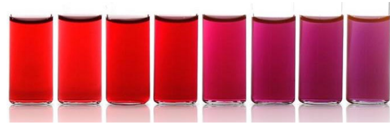
Figure. Gold nanoparticles of different diameters in solution
