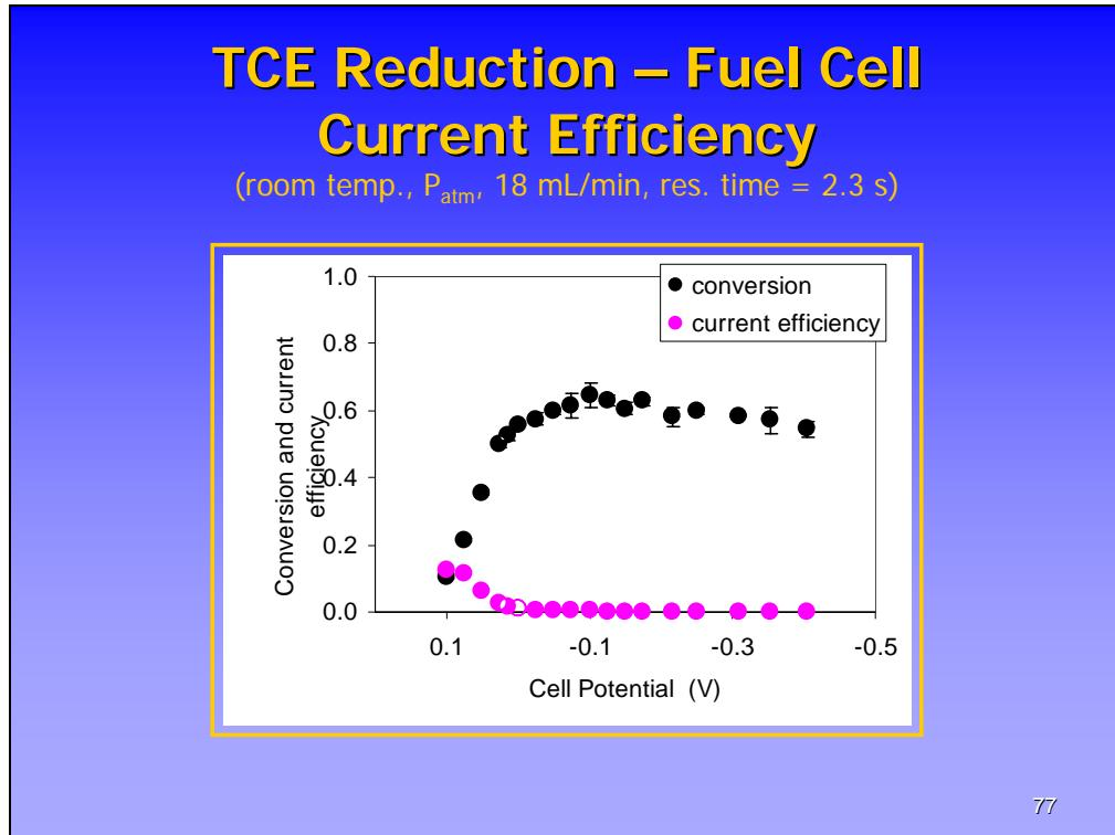
Here in this graph the current efficiency was plotted with respect to cell potential, and TCE conversion was also plotted. Current efficiency here is defined as the ratio of the current used for TCE reduction to total current. As you can see, the current efficiency is relatively low due to large amount of hydrogen generated.
