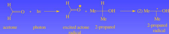
Acetone in its excited state, extracts a hydrogen atom from a suitable donor, such as 2-propanol, producing a highly reduced 2-propanol radical that is capable of reducing a variety of halogenated targets.
