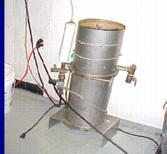
Water Treatment Unit (above) Treats separator water
