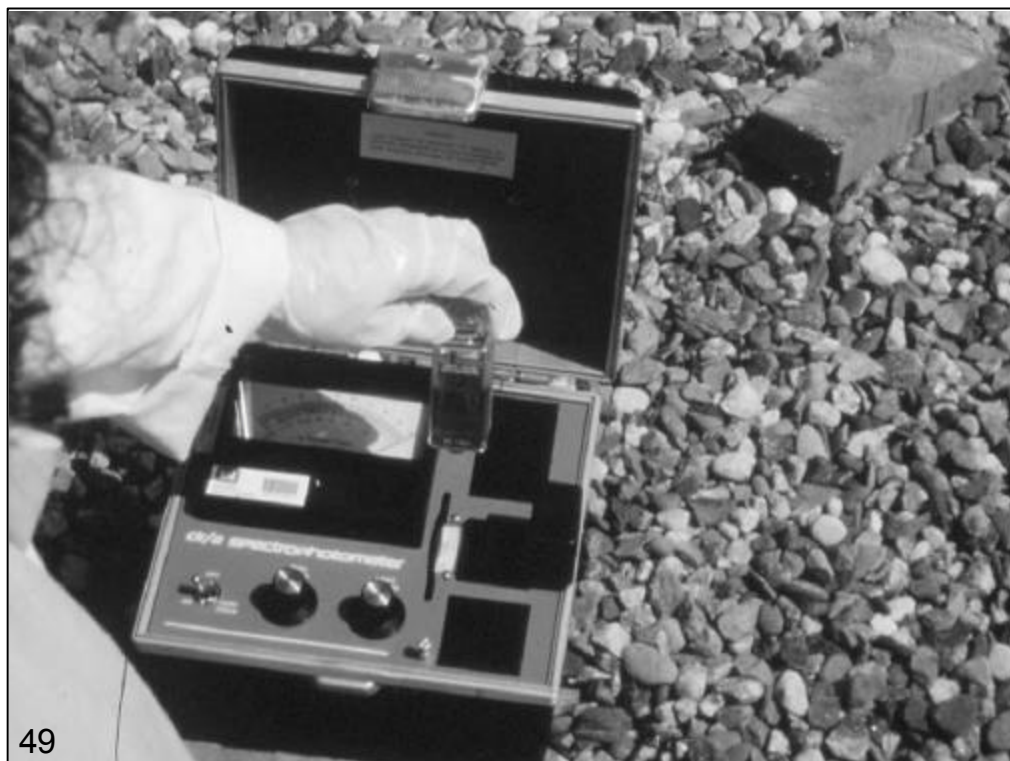
Closer view of spectrophotometer and reddish colored solution that forms after addition of reagents to soil extract when TNT is present.
