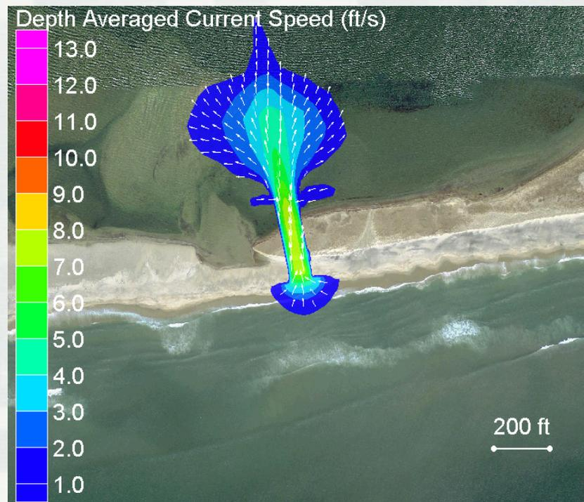
Maximum depth-averaged current velocity during flood tide.
