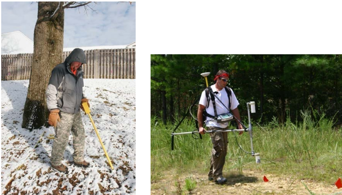
Figure 6-1: Schonstedt GA-52 (left) Fluxgate Magnetometer and Geometrics G-858 (right) Optically Pumped Metal Detector
