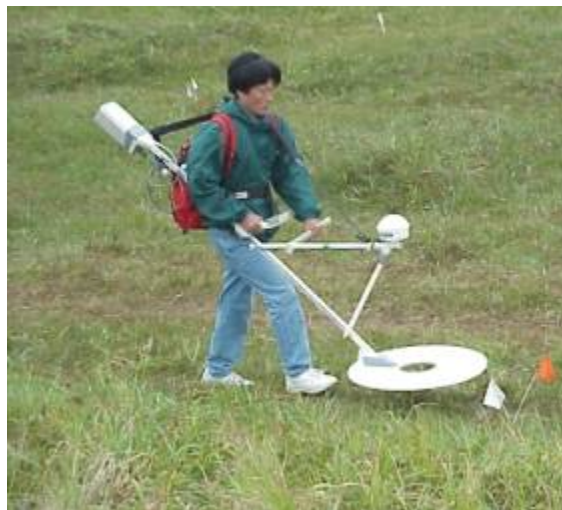
Figure 6-4: Geophex GEM-3 FDEMI Sensor
