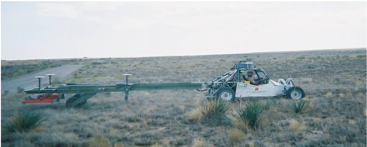
Figure 6-27: Example of a Multiple Instrument Array
