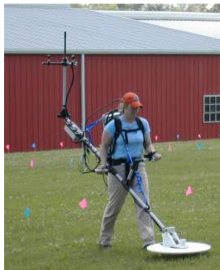
Figure 6-26: Example of a Man-Portable Geophysical System
