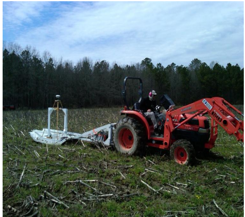
Figure A-9. MetalMapper in use at Camp Sibert Site 18
