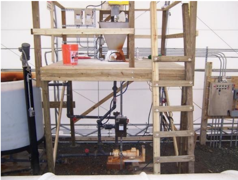
Figure 5. Funnel and grinder pump for mixing water with quicklime and recirculating back to the neutralization/mixing tank (left-side of photo).
