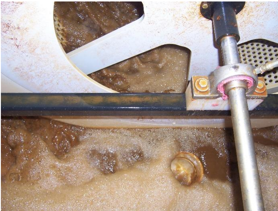
Figure 6. RCTS™ unit with orange/rust colored discharge water.
