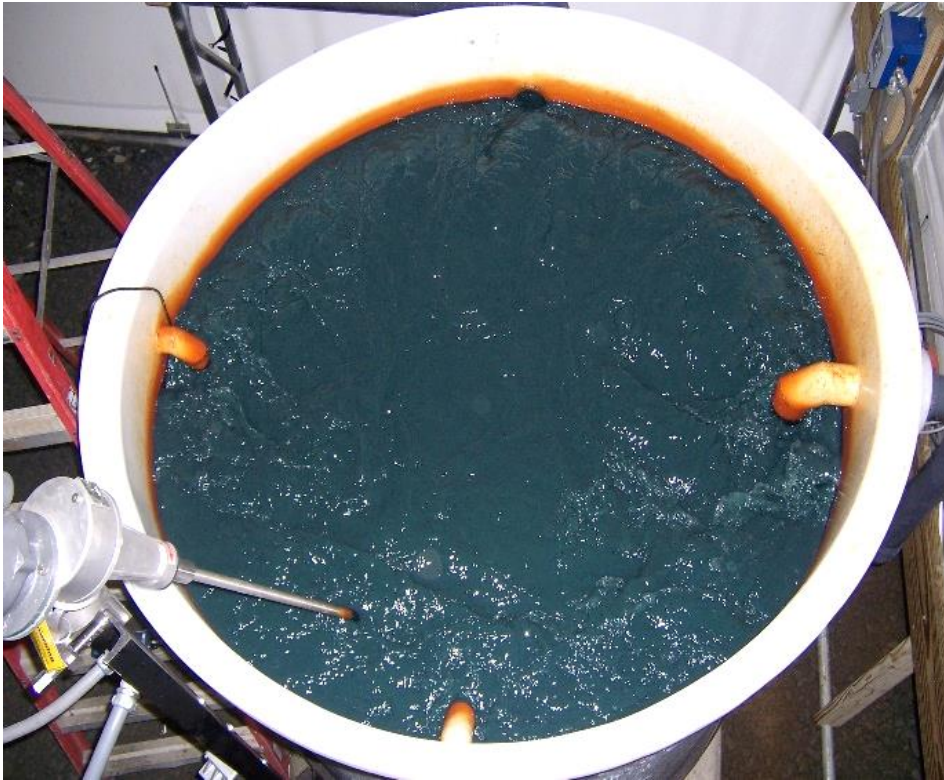
Figure 4. Neutralization/mixing tank with dark blue-green color of ferrous hydroxide particles.
