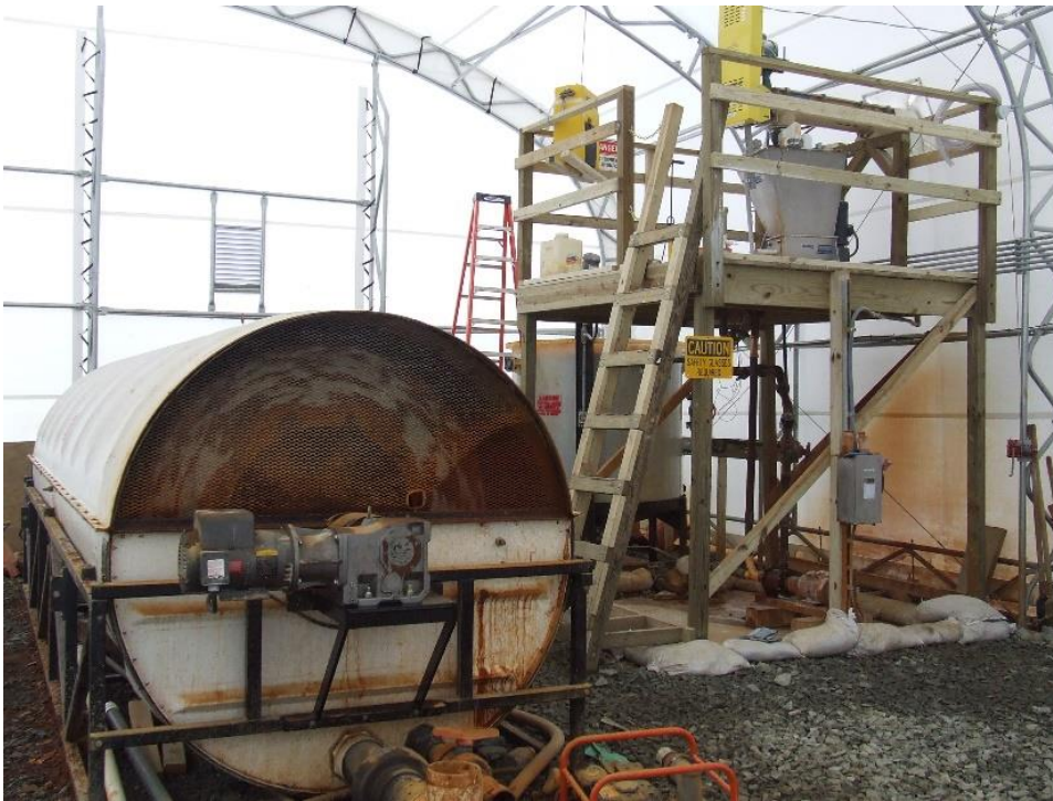
Figure 7. Layout inside building: RCTS™ unit on left hand side; funnel, grinder pump, and recirculation plumbing on right-hand side; neutralization tank right-hand side at back.
