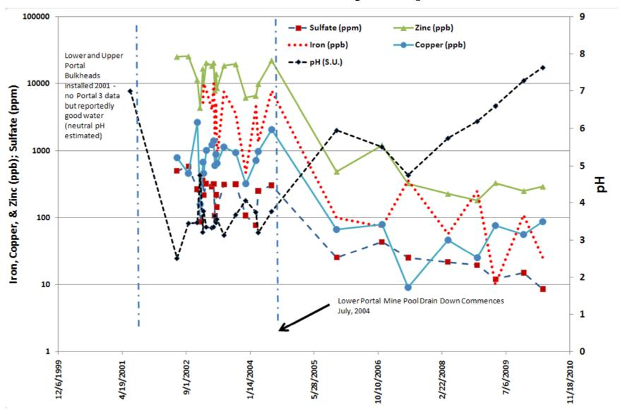
0.07 to 0.11 gpm of Lower Portal MIW satisfies metal load in Portal 3 based on sulfate, zinc, and copper
