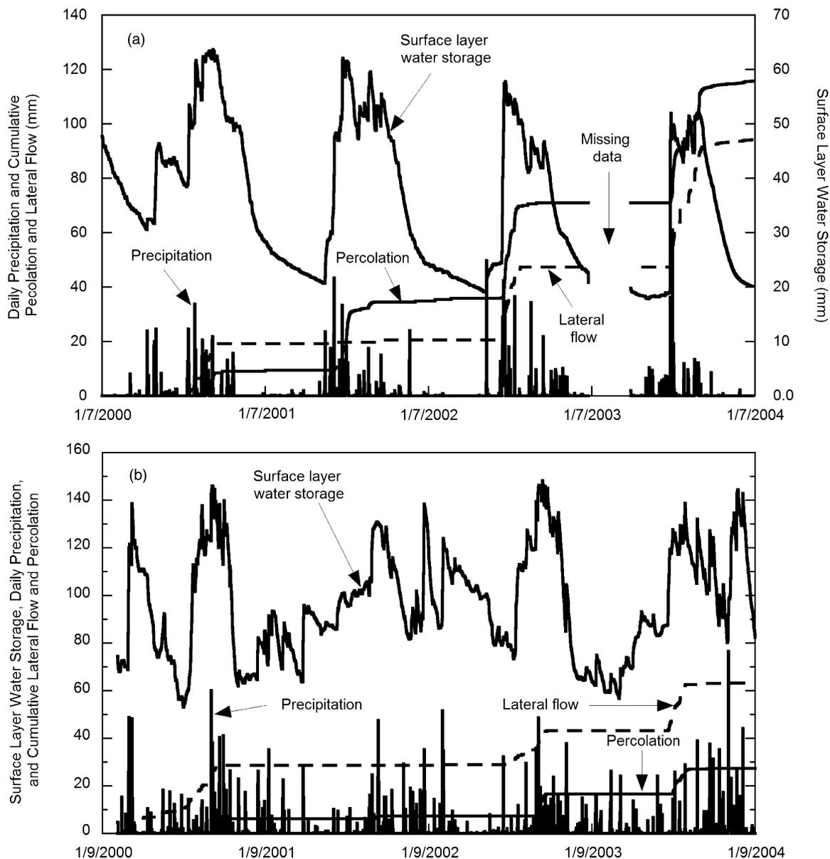
**Fig. 8.** Water balance components for the test sections at (a) Marina, California, and (b) Omaha, Nebraska (percolation coincides with increased water storage in the surface soil layer and lateral flow on the barrier geomembrane; the very high rate of percolation at Marina is probably a result of damage to the geomembrane during installation)
