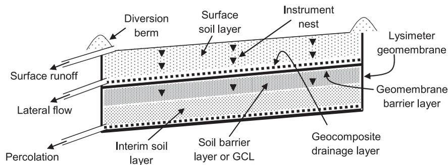
Fig. 3. Schematic of ACAP lysimeter for composite covers
