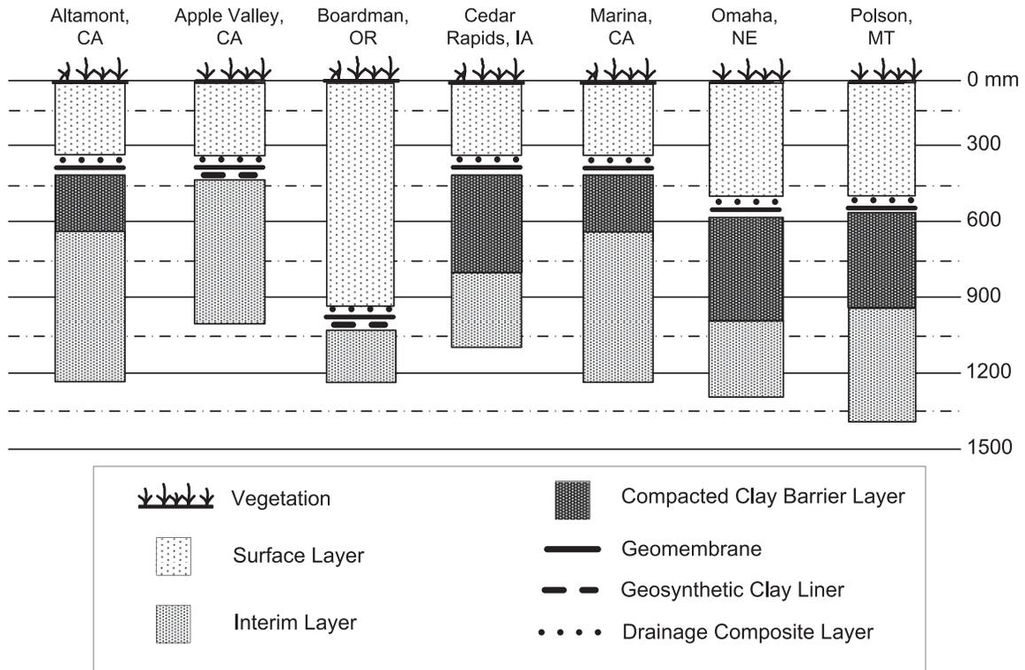
Fig. 2. Profiles of ACAP composite covers
