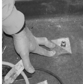
Figure D-4. Installation of subslab soil gas sample port. Courtesy Kansas Department of Health and Environment
