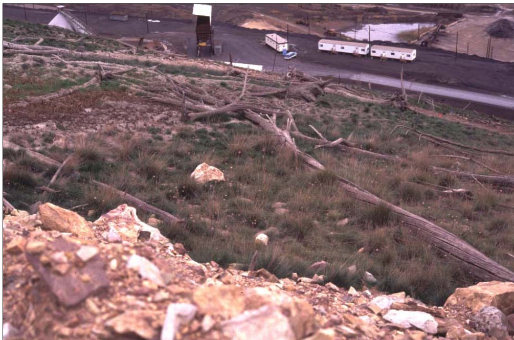
Palmerton, PA, 1990: Oyler's First Test Plot Using Biosolids + FlyAsh + Limestone, with 'Merlin' Red Fescue; adjacent control.
