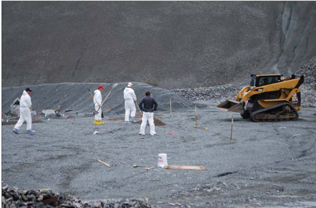
August 24, 2011: Applying the compost mixtures to test plots; compost was raked even, then seeded with crop mix.
