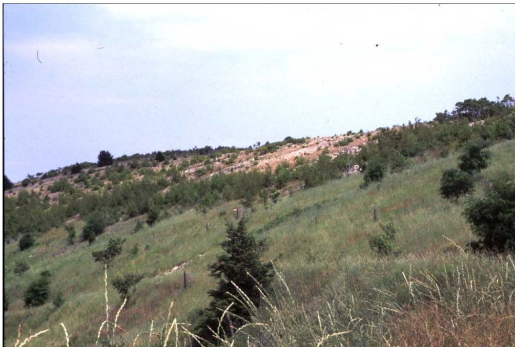
Palmerton, PA: Blue Mountain – 1999; Foreground = Biosolids+Limestone+FlyAsh; Background = untreated Control
