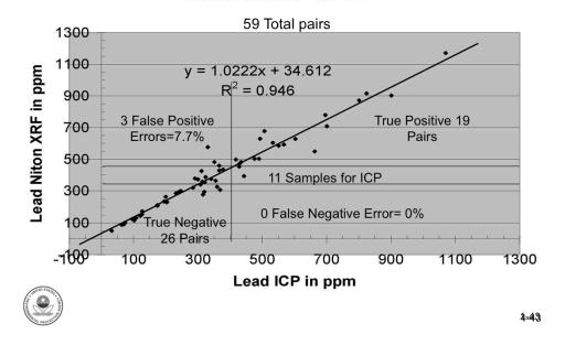
Structure of a 3 way decision. 19 true positives, 26 true negatives, 3 false positives, and 11 samples for ICP. Region of uncertainty is 350-450 ppm. Below 350 is definitely clean, above 450 is definitely dirty (with 5% false positives)
