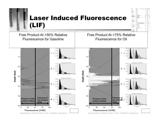
Fuels (PAHs) in the vadose and saturated zones (>50-100 ppm, free product) Excitation sources- lasers (single wavelength, tunable), Hg lamp (FFD or exsitu)
