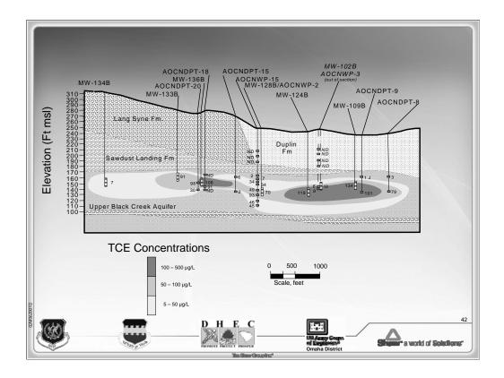
E--W Section shows TCE plume dominate transport is between 160 to 140 ft MSL. Apparent dissection of the plume is due to flow pattern in and out the line of section.
