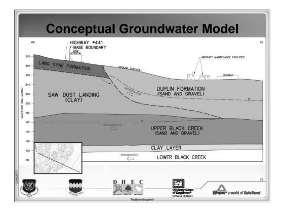
Inset shows line of section. Perpendicular to topographic gradient and structural grain, and crosses the run ways
