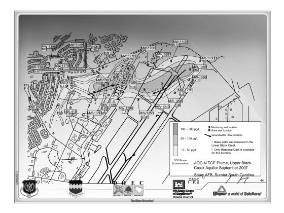
The plume in the Upper was characterized using the real-time measurements in the runway and maintenance building areas, however, because of the difficult geological conditions to the west, profiling and DPT sampling to over 150 feet was not possible. But based on the data available the plume migrating pathway could be projected and the final well locations were cited based on the projections.
