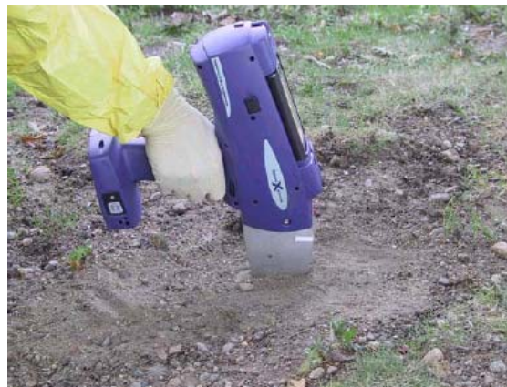
Figure 6-1. Innov-X XT400 XRF analyzer set up for portable in situ analysis.
